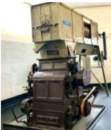
The Seck mill, open squares at Unicorn to be superseded by 20hL dual purpose vessels at Bredbury
