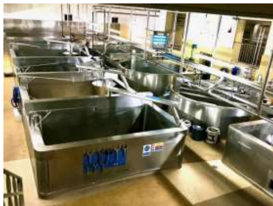
The Seck mill, open squares at Unicorn to be superseded by 20hL dual purpose vessels at Bredbury
