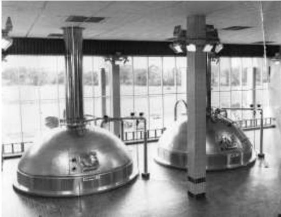
The Berkshire Brewery at Worton Grange by the M4 motorway in Reading operated only from 1980 until 2010. On the left are a pair of 800bbl coppers, one of 22 x 1540 bbl conical fermenters and a keg line.
