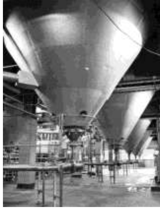
The Berkshire Brewery at Worton Grange by the M4 motorway in Reading operated only from 1980 until 2010. On the left are a pair of 800bbl coppers, one of 22 x 1540 bbl conical fermenters and a keg line.
